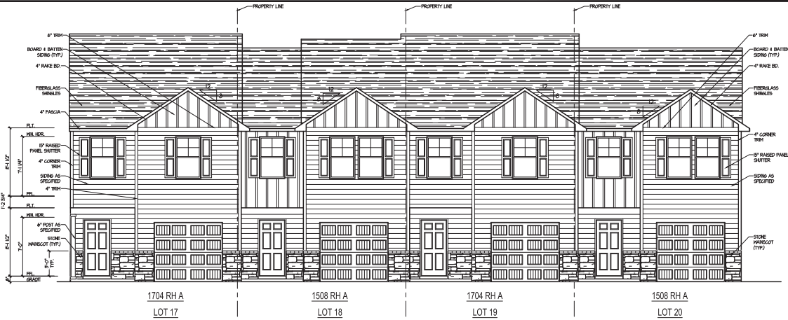
FRONT ELEVATION 4 UNIT BUILDING
